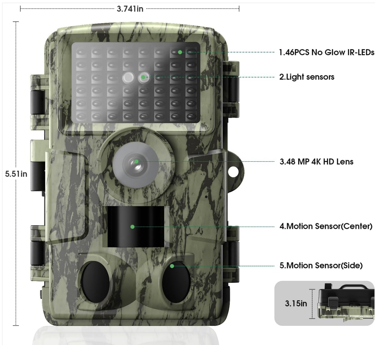
Image 3.1: Camera Components and Dimensions
