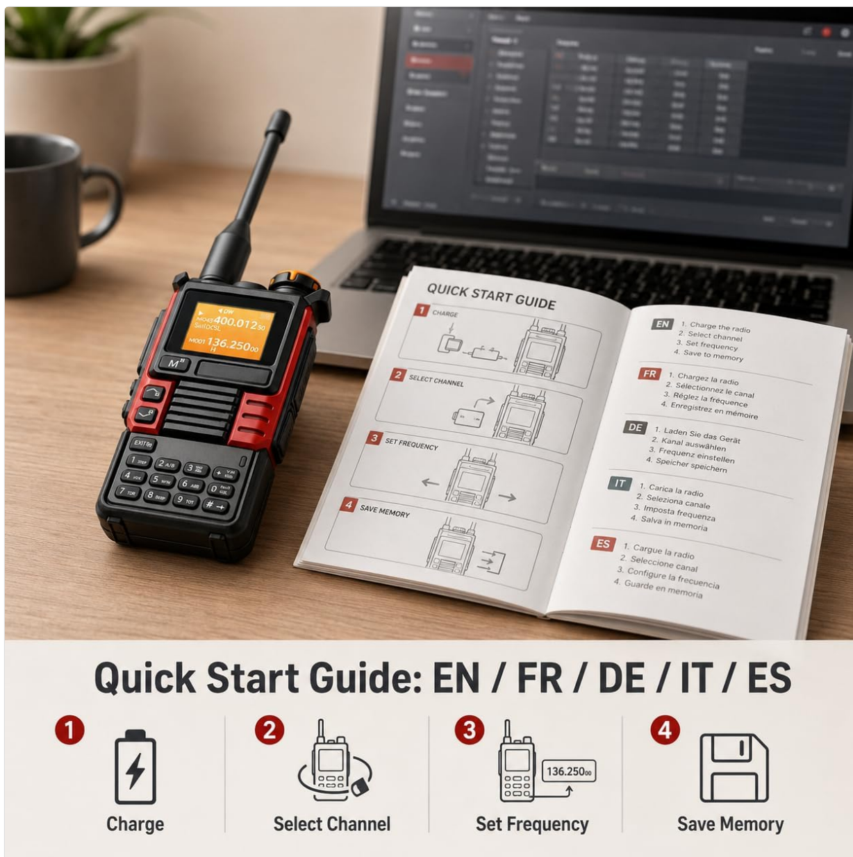
Figure 3.3.1: Quick Start Guide illustrating the initial steps: Charge, Select Channel, Set Frequency, and Save Memory.
