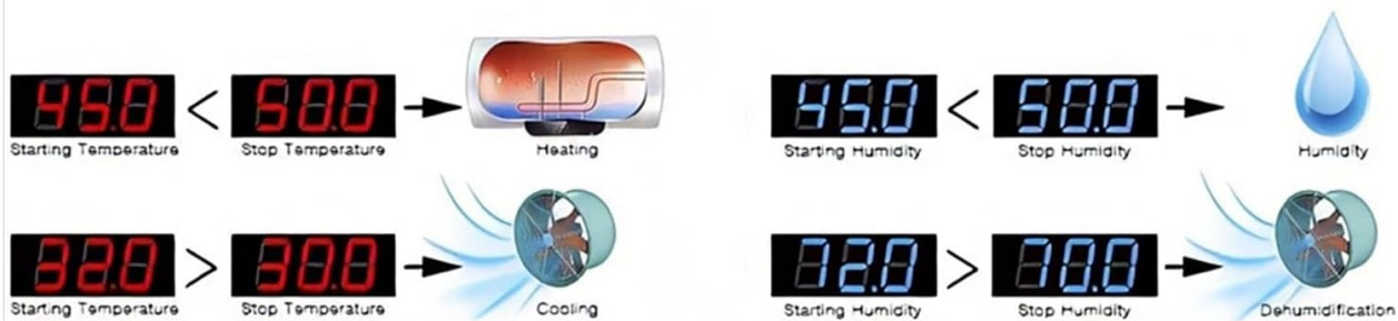
Image 5.1: Visual guide for setting the startup and stop temperatures and humidity levels on the STC-3028 controller, including examples for heating, cooling, humidification, and dehumidification.
