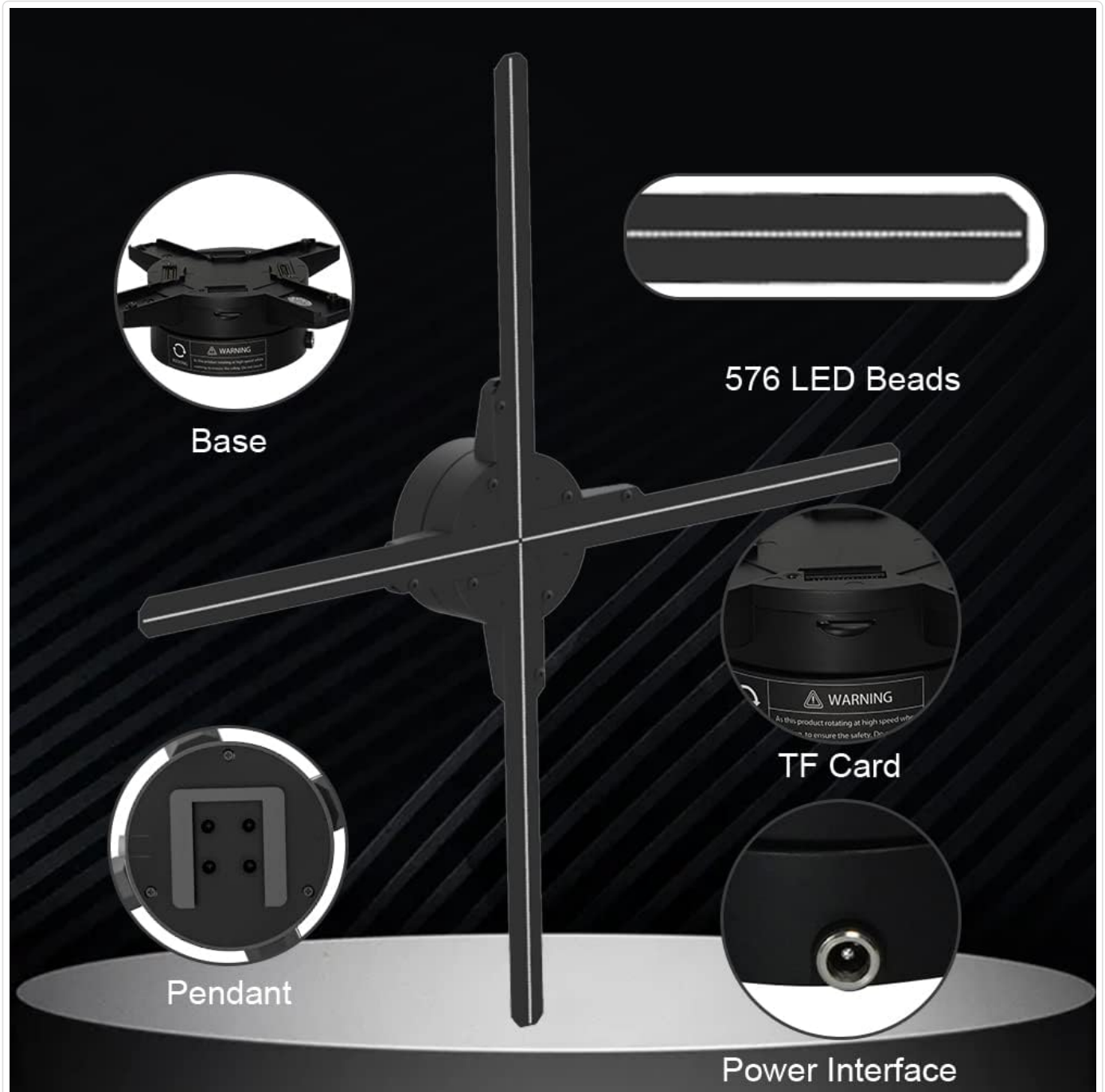
Figure 2: Main components of the hologram fan.
