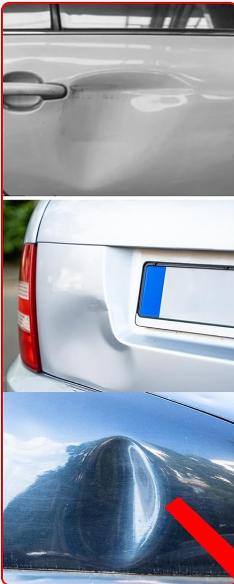
Figure 4.2: Illustrates the types of dents that are suitable for repair with the PDR100 tool. It is primarily effective for soft and smooth dents that do not extend to the edge of the panel. Examples of suitable and unsuitable dents are shown.
