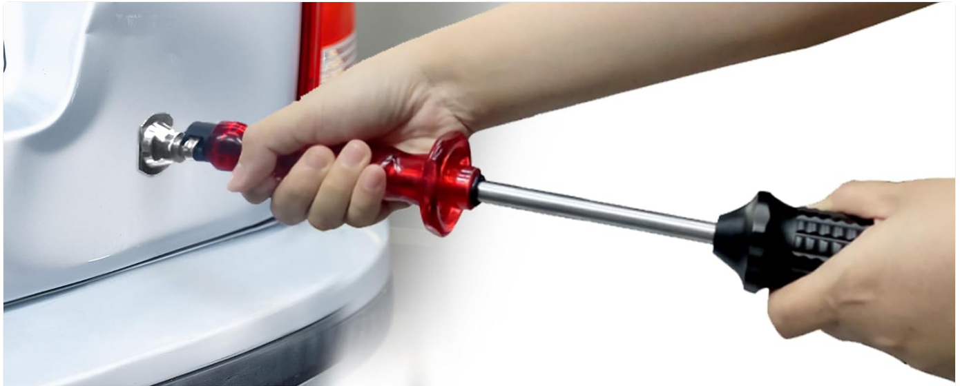
Figure 3.1: The WOYO slide hammer puller with various steel tabs and an adapter connector. The handle is designed for increased friction and comfortable grip.
