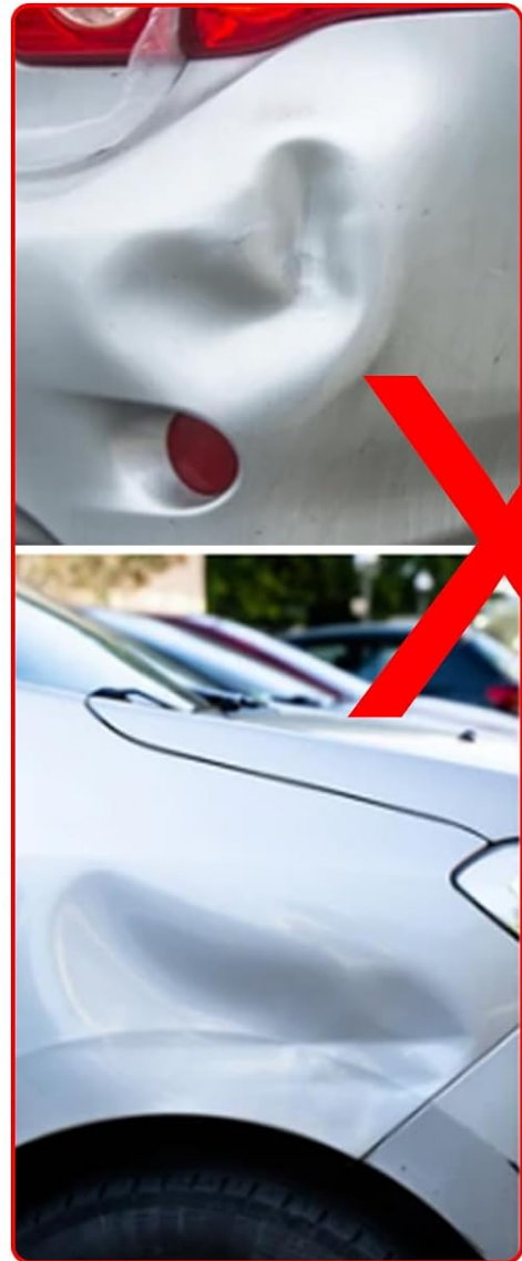
Figure 4.2: Illustrates the types of dents that are suitable for repair with the PDR100 tool. It is primarily effective for soft and smooth dents that do not extend to the edge of the panel. Examples of suitable and unsuitable dents are shown.
