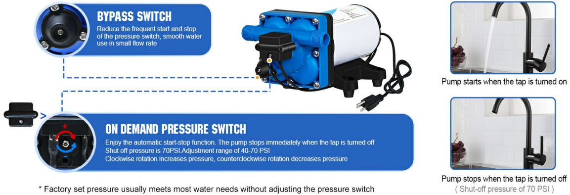
Image: Explanation of the bypass switch for smooth water use and the on-demand pressure switch with adjustable shut-off pressure (40-70 PSI).
