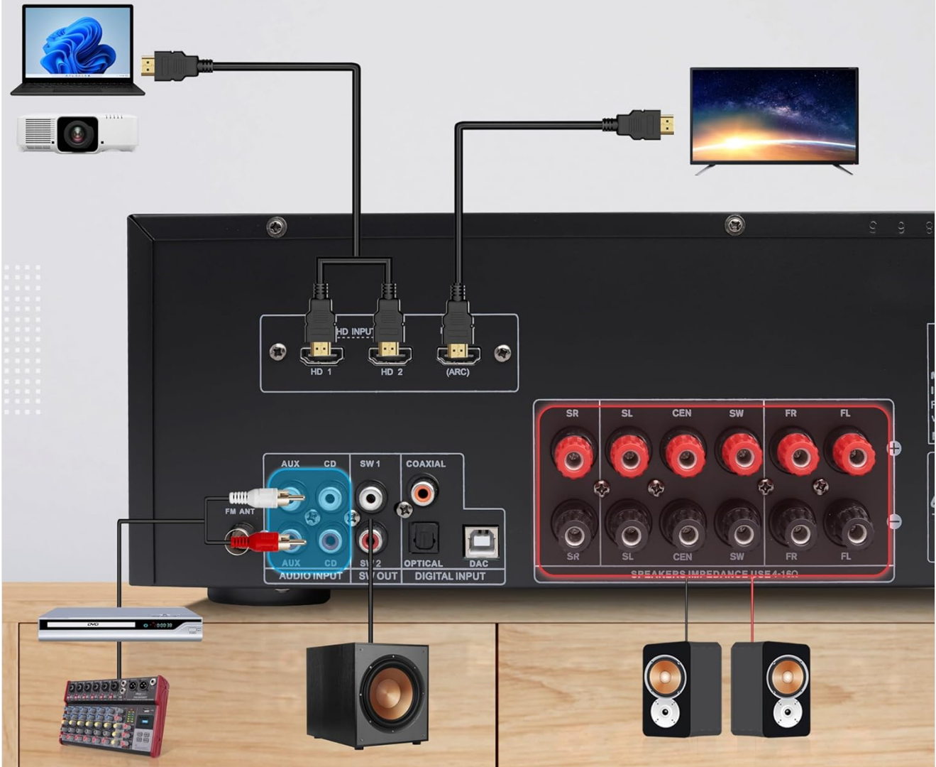
Image: An illustration demonstrating how to connect various devices like laptops, projectors, TVs, DVD players, subwoofers, and speakers to the Pyle PT865BT receiver's rear panel inputs and outputs.
