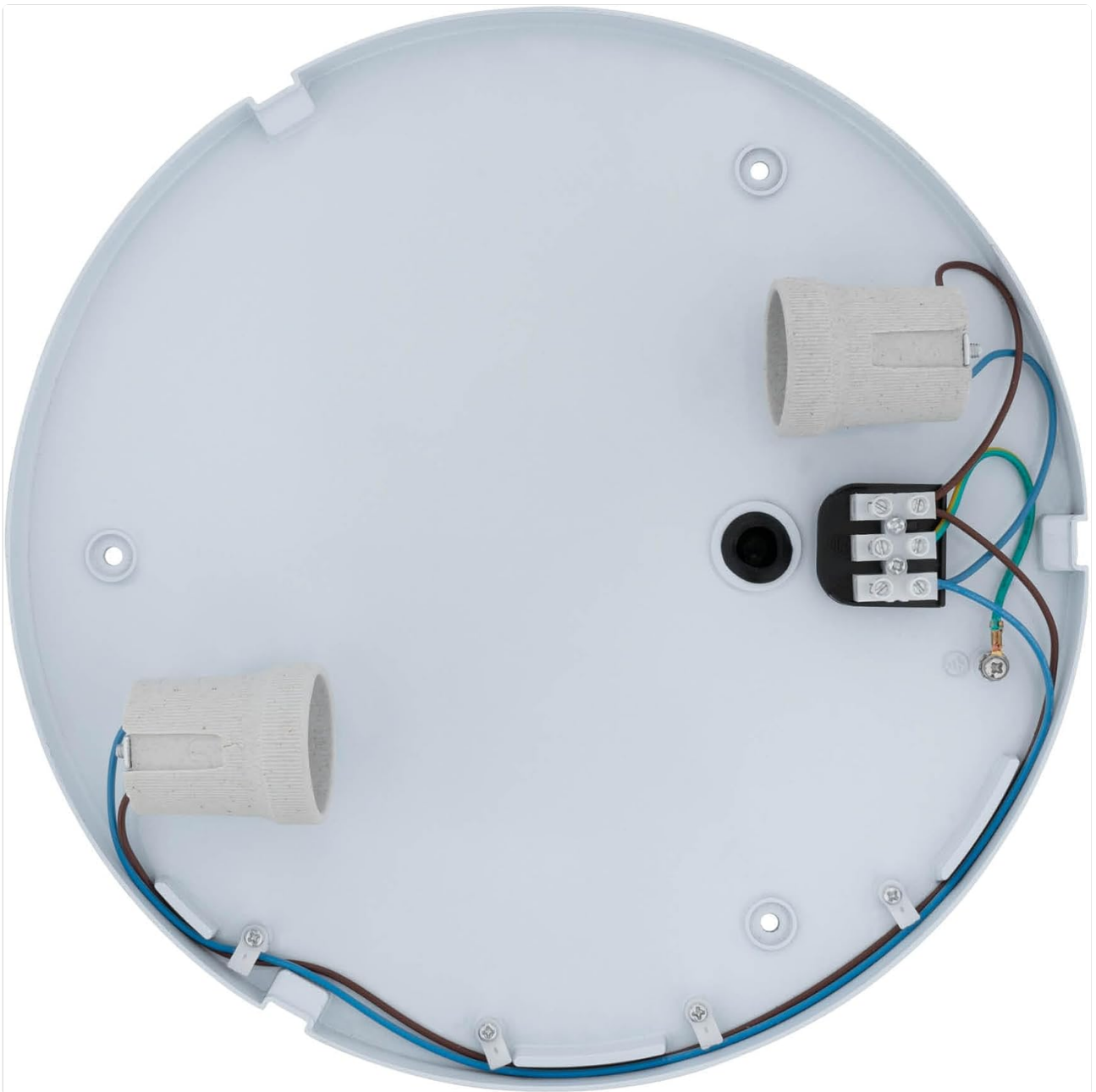
Image: Internal wiring and E27 sockets. This image shows the two E27 bulb holders and the electrical terminal block for connecting the main power supply.
