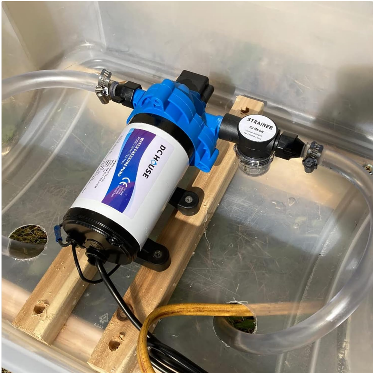
Image 5.1: Example installation of the water pump with an inline filter.
