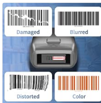
Image: Examples of different barcode conditions that the scanner can read, including damaged, blurred, distorted, and color barcodes.
