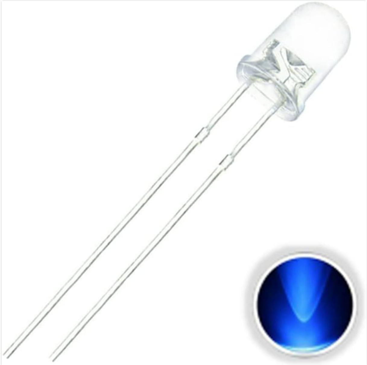
Image 1: A single 5mm blue LED diode. Note the clear lens and the two metal leads extending from the bottom. The longer lead is the anode (+), and the shorter lead is the cathode (-).
