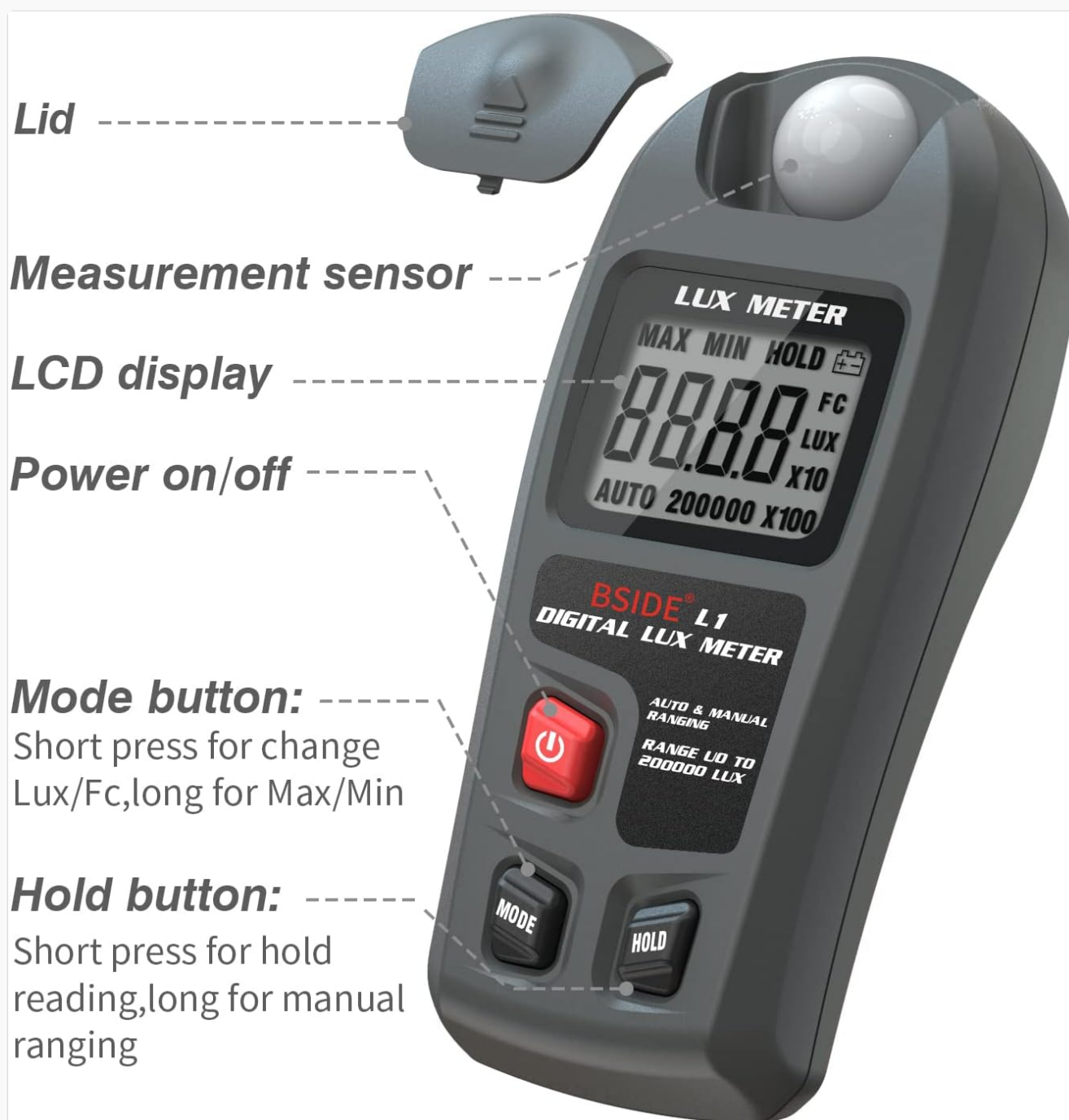
Figure 2: Labeled components of the BSIDE L1 Digital Lux Meter.
