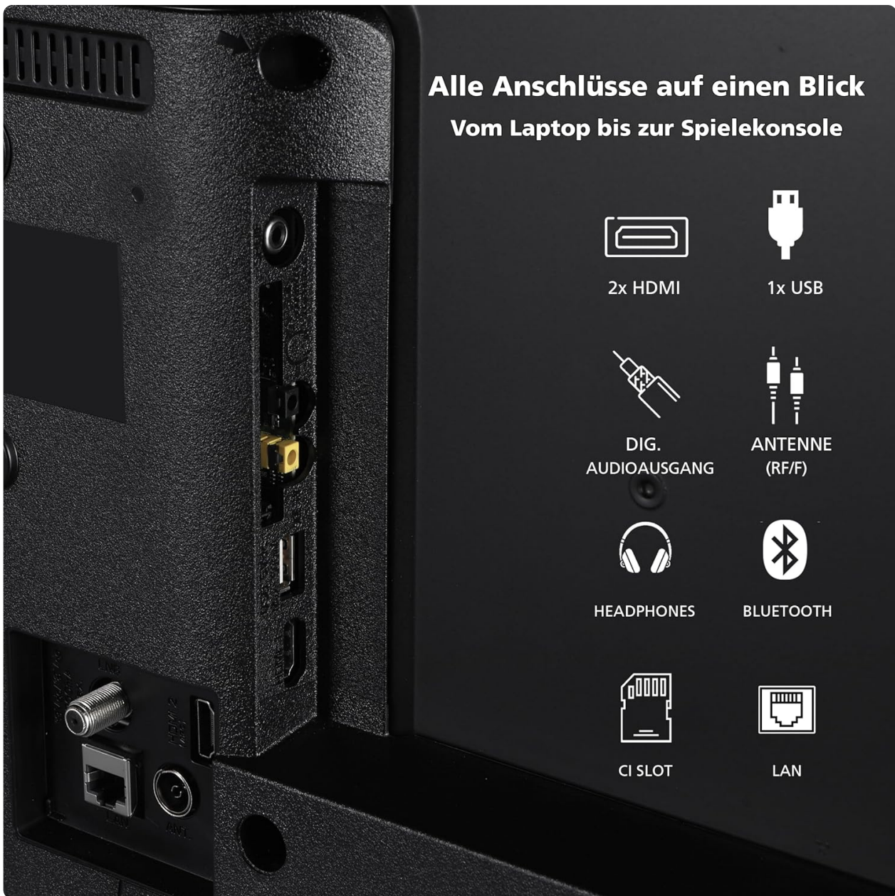
Image: Close-up view of the rear panel of the JVC LT-32VAF3355 TV, highlighting all available connection ports including 2x HDMI, 1x USB, Digital Audio Out, Antenna (RF/F), Headphones, Bluetooth, CI Slot, and LAN.
