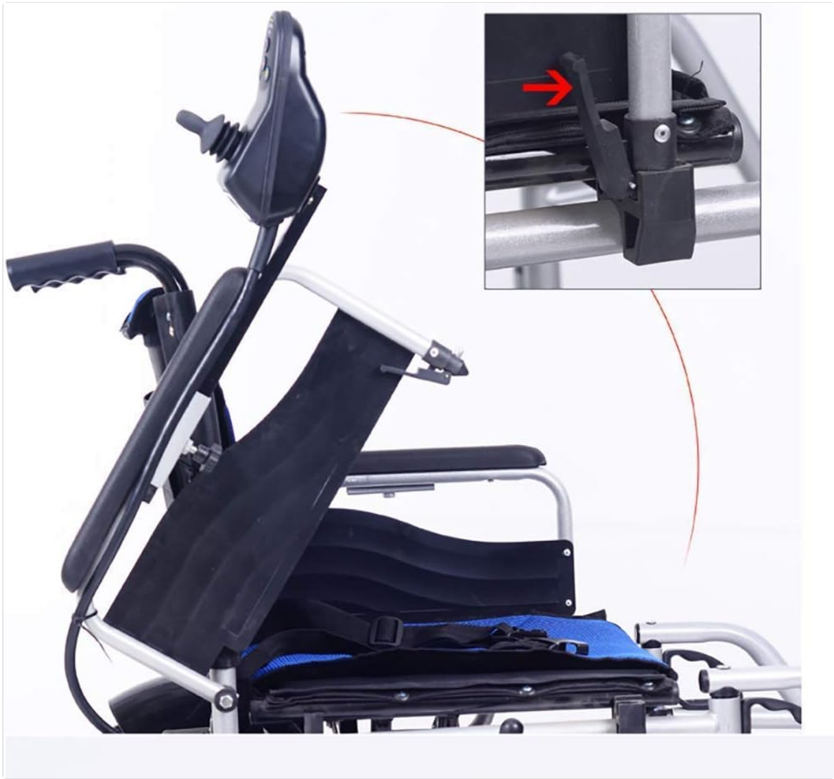
Figure 3: Close-up view of the latch mechanism used to secure the wheelchair frame in its unfolded position. An arrow indicates the latch.
