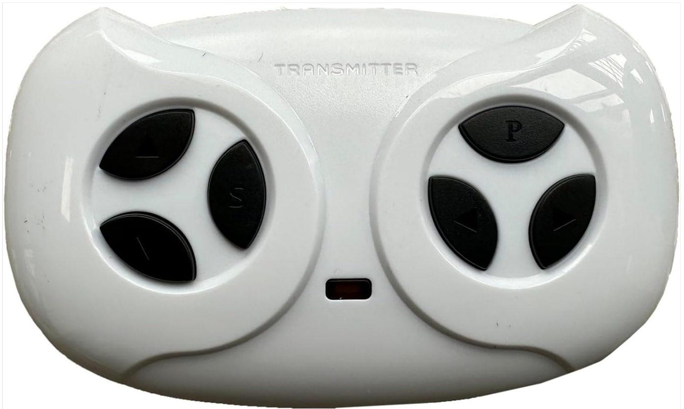
Figure 1: Front view of the JR1602FCC Remote Control. It is white with two circular control pads, each containing three black buttons. The left pad has buttons for forward, speed, and back. The right pad has buttons for brake, right, and left. A small red indicator light is visible below the "TRANSMITTER" label.
