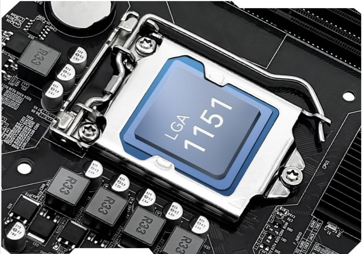
Image 2.1: Detailed view of the Intel LGA 1151 CPU socket on the H110 motherboard.
