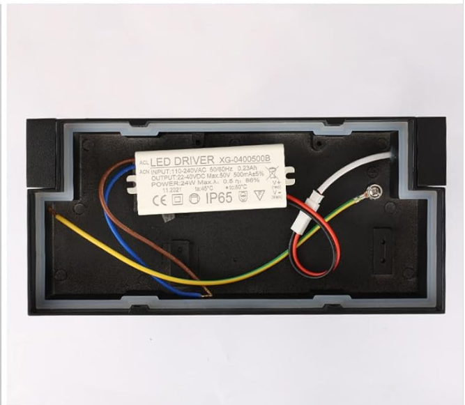
Inside IP65 LED Driver
