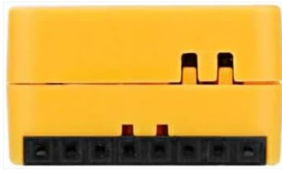
Figure 4: Side view of the M5StickC PLUS2, indicating the location of the power button (Button C).
