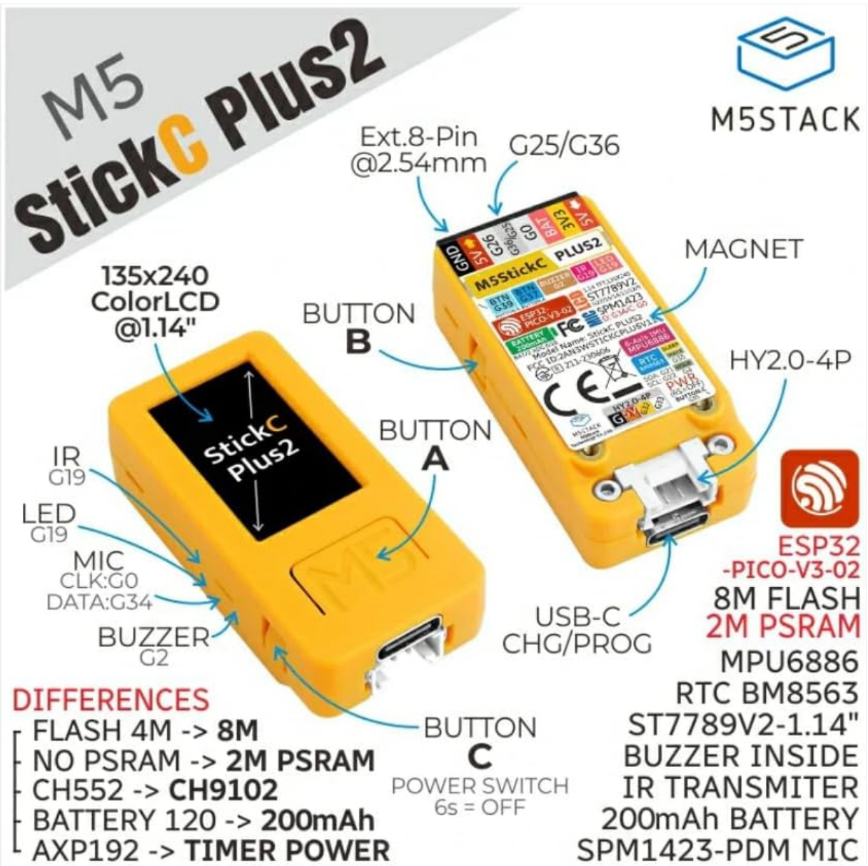
Figure 2: Top view of the M5StickC PLUS2, illustrating the pinout for the external header and labels for internal components like the ESP32 chip, display driver, and battery.
