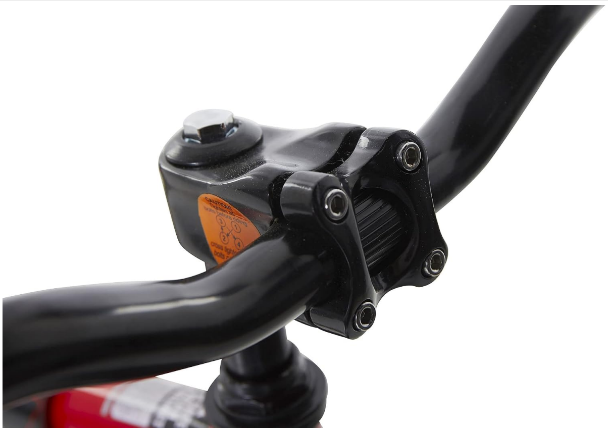
Figure 2: Close-up of the handlebars and stem, which require attachment during initial setup.
