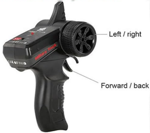
Image: Remote control diagram illustrating proportional throttle and steering functions.
