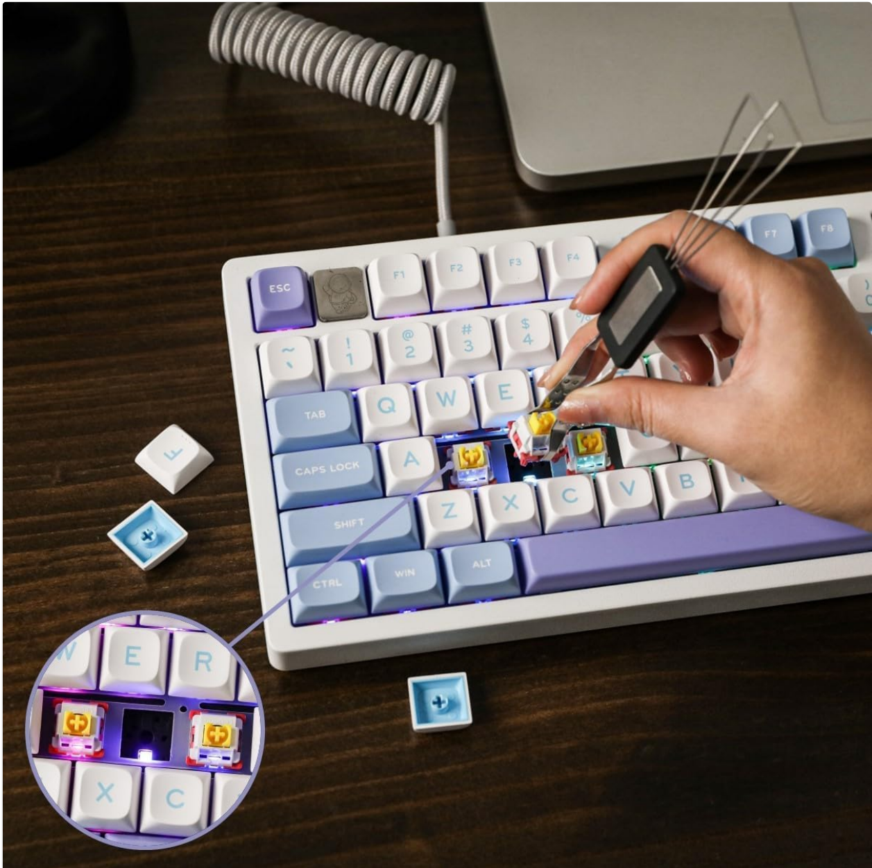
Figure 6: Demonstration of replacing hot-swappable switches.
