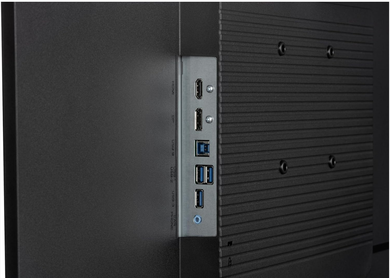
Image: Close-up view of the monitor's input ports, including HDMI, DisplayPort, USB-A, USB-C, and audio output. These ports allow for various connectivity options.
