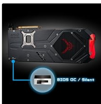
Figure 3.6: Dual BIOS switch for selecting between OC (Overclocking) and Silent modes.
