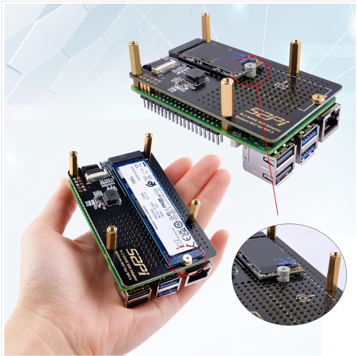
Image: Installation of an M.2 NVMe SSD onto the N07 peripheral board, showing the use of a screw to secure the SSD.
