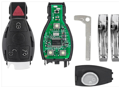
Figure 2.5: Exploded view of the key fob, showing the outer casing, circuit board, emergency key, and battery compartment.
