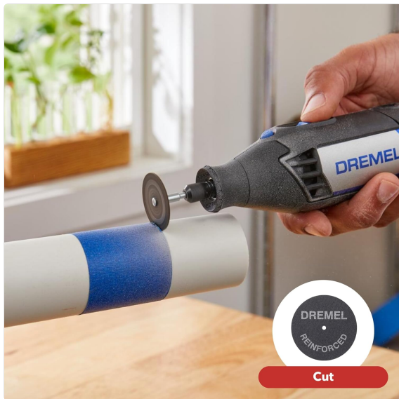
Image 6.1: Using the Dremel 4000 with a cutting wheel on a PVC pipe.
