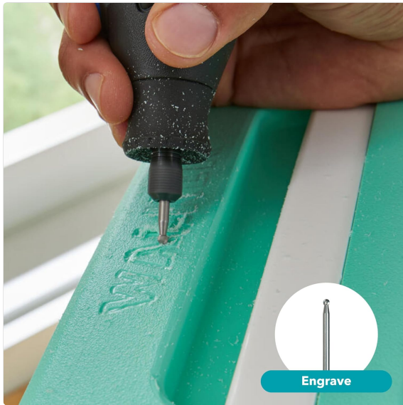
Image 6.3: Engraving a pattern onto a plastic surface using a Dremel tool.
