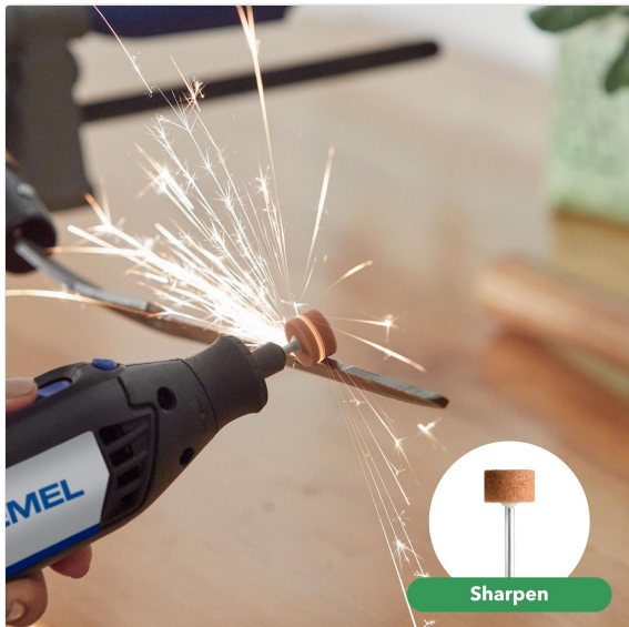
Image 6.4: Sharpening a metal blade with a Dremel rotary tool and grinding stone.
