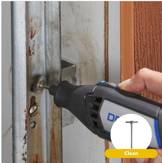
Image 6.5: Cleaning a rusty metal door hinge with a Dremel tool and wire brush accessory.
