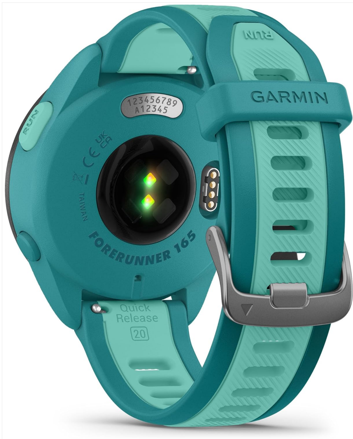
Image: The back of the Garmin Forerunner 165 Music smartwatch, highlighting the optical heart rate sensor and the charging contacts. The model number "FORERUNNER 165" is visible.
