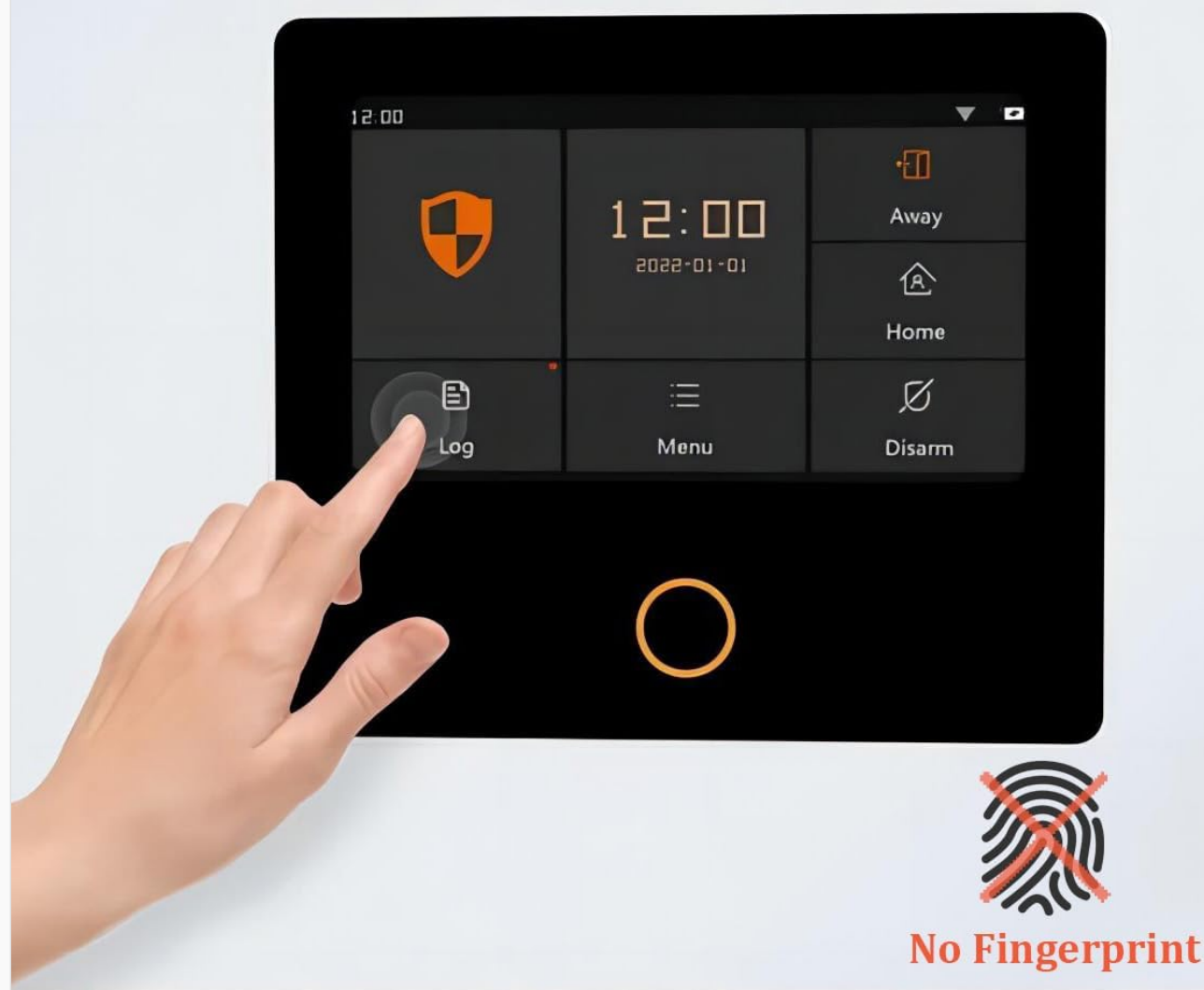
Figure 5.1.1: The 4.3-inch touch screen panel provides a user-friendly interface for system control.
