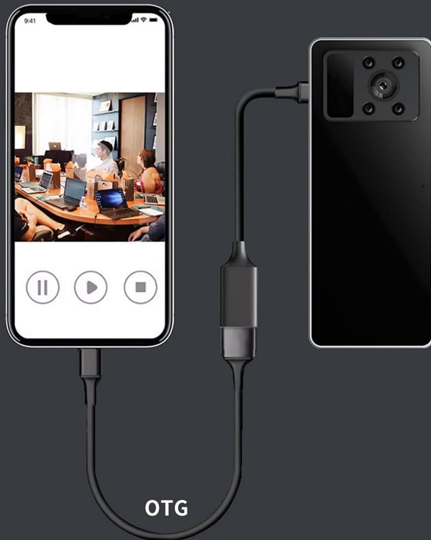
Figure 6: Connecting the camera to a smartphone using an OTG cable for video playback and file management.
