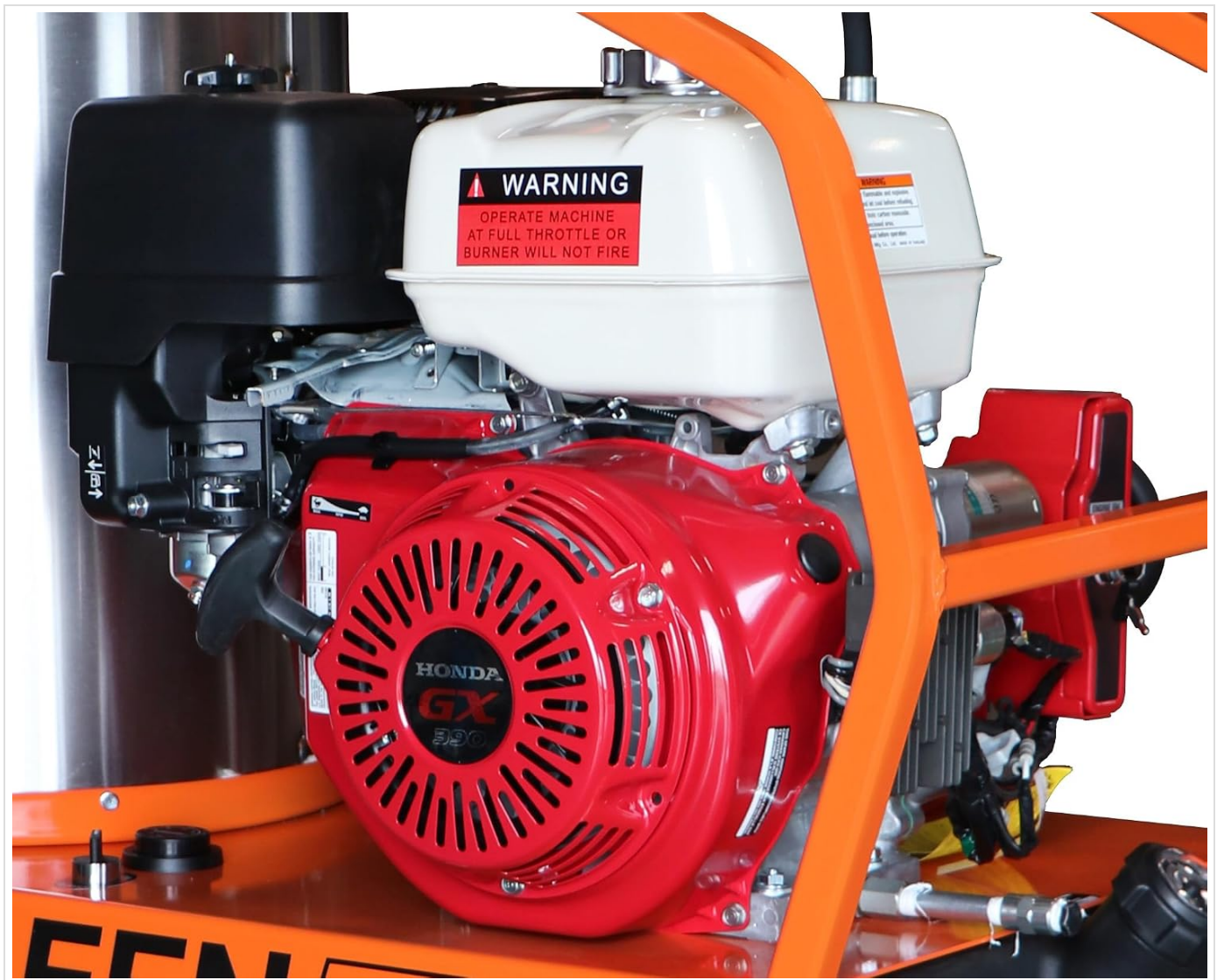
Image: Close-up view of the 13 HP Honda GX engine, which powers the pressure washer. Note the warning label regarding operation at full throttle.
