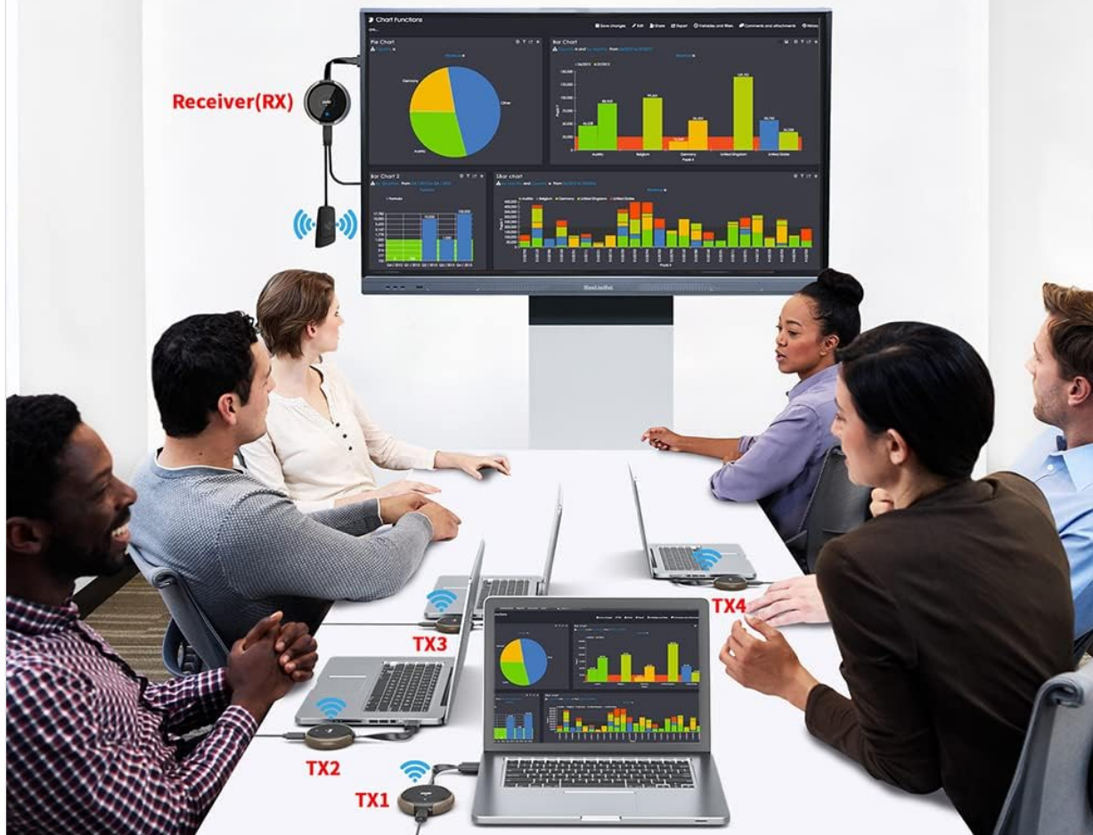
Image 5: A diagram illustrating a "Switch Mode" setup where one Receiver (RX) is connected to a large display, and multiple Transmitters (TX1-TX4) are connected to individual laptops. Users can switch which laptop's display is shown on the main screen.
