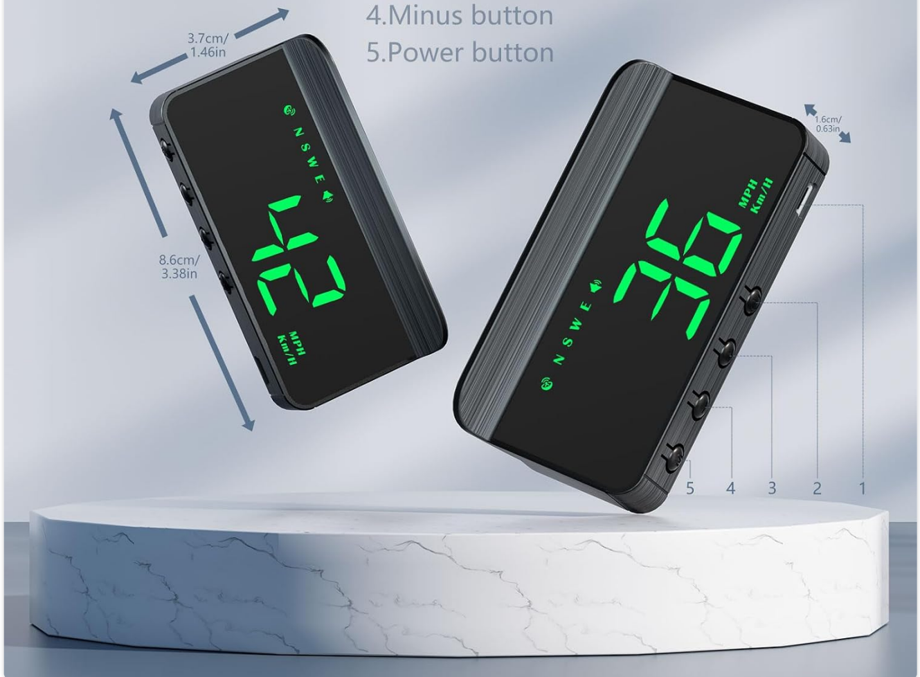
Figure 9: M1 HUD product presentation with dimensions and button layout.
