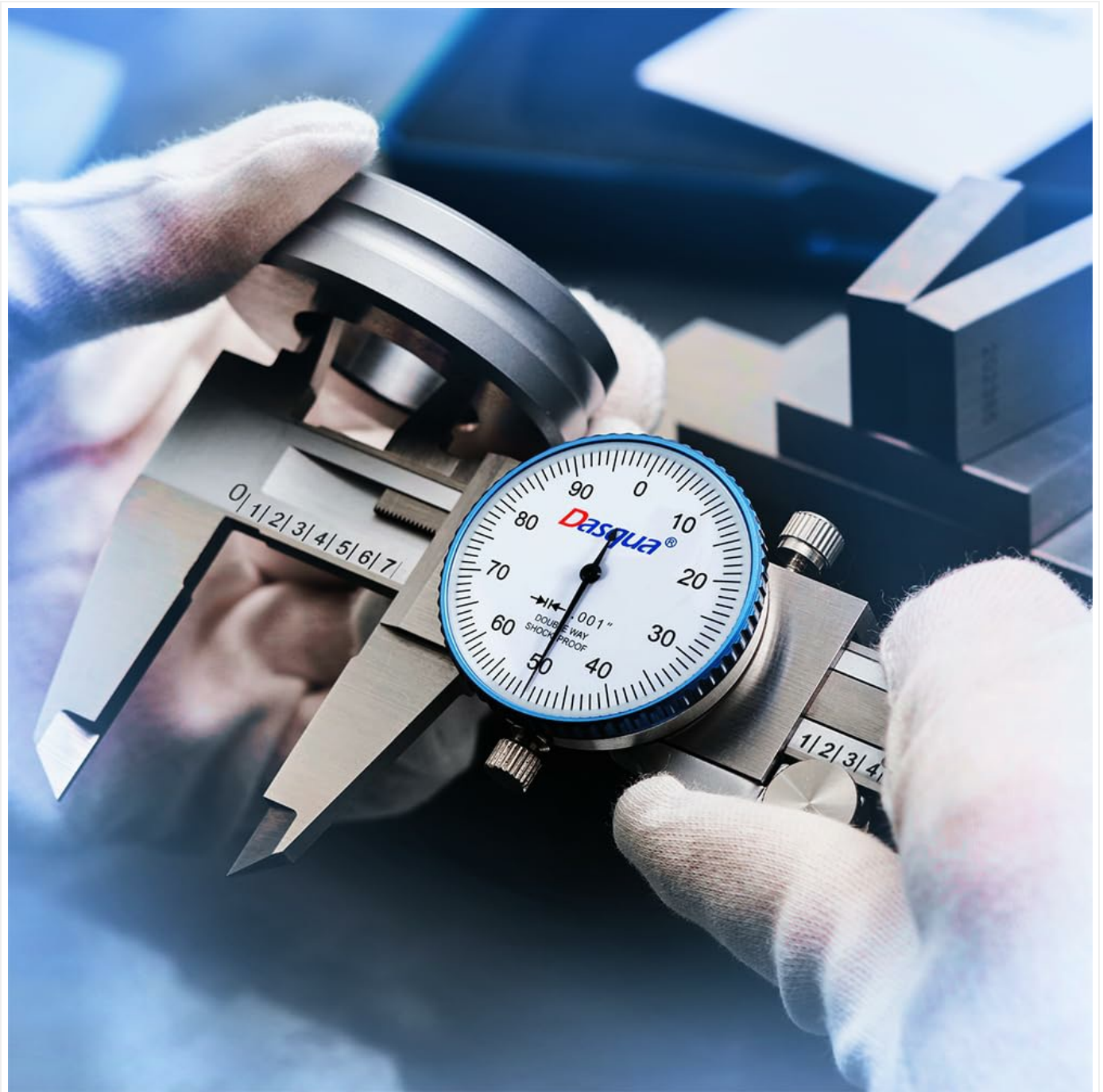
Figure 5: Measuring an object's external dimension with the caliper.
