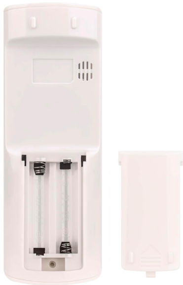
Figure 2.4: Rear view of the remote control with the battery compartment cover removed, showing the slots for two AAA batteries.
