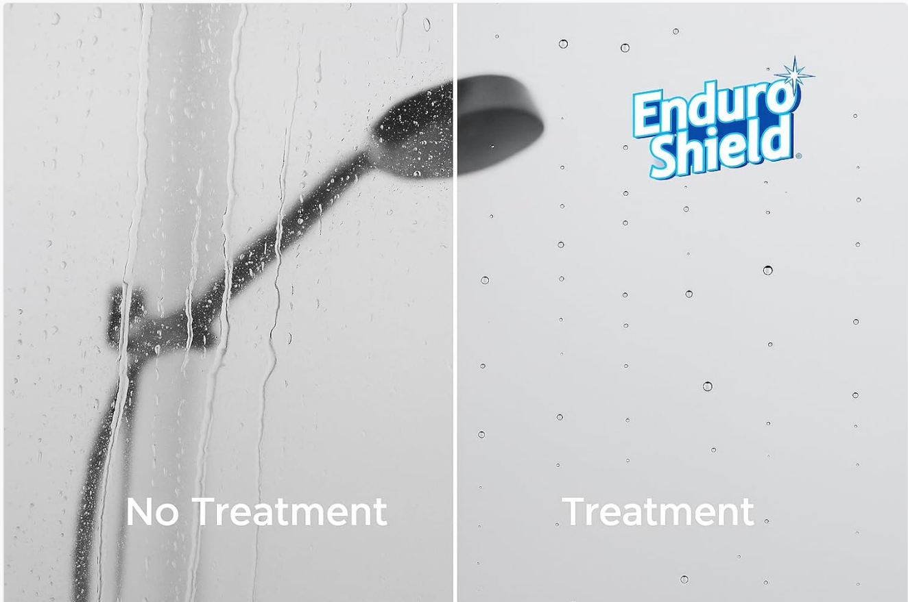
Figure 4: Visual comparison of EnduroShield treated versus untreated glass.
