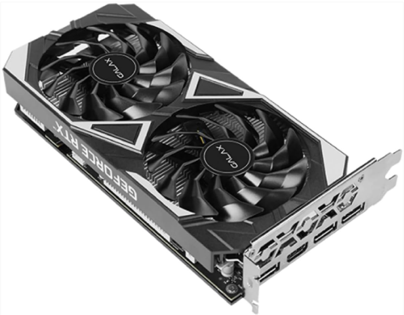
Image: Rear view of the graphics card, highlighting the DisplayPort and HDMI output connectors.
