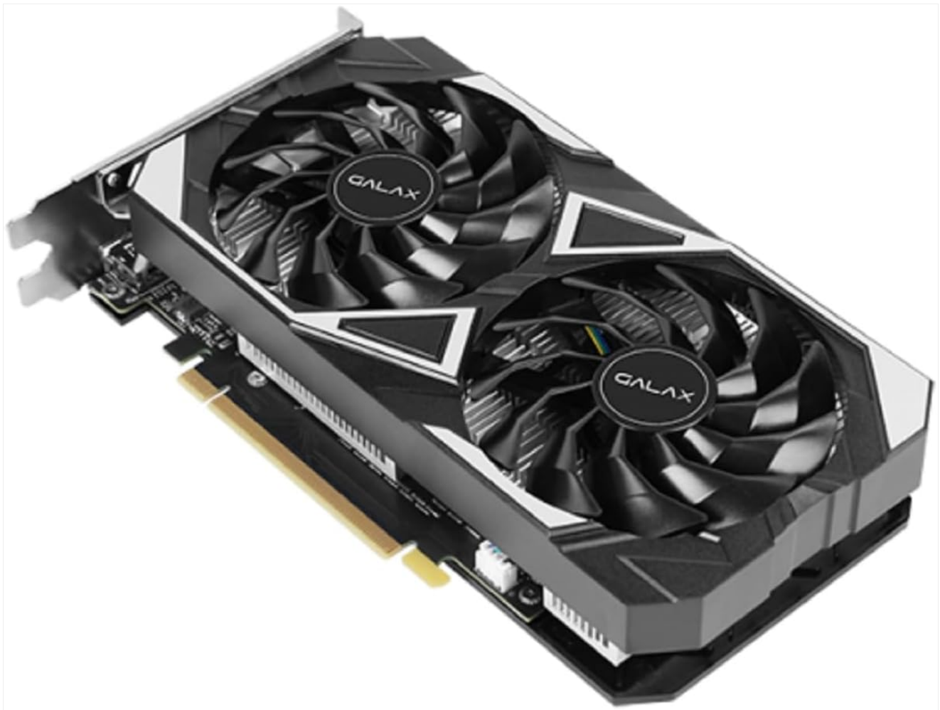
Image: The Galax RTX 3050 EX graphics card, illustrating its dual-fan design and PCI-Express interface for installation.
