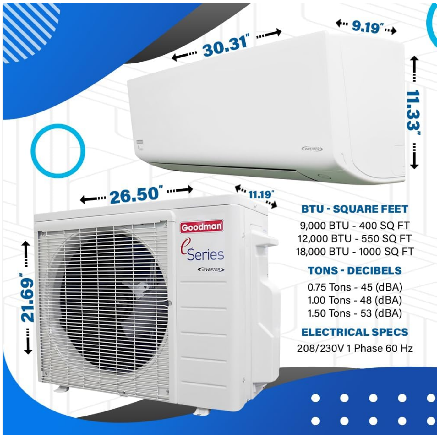
Figure 4: Dimensional specifications and performance ratings for the Goodman Mini-Split AC/Heating System, including BTU, square footage coverage, and noise levels.
