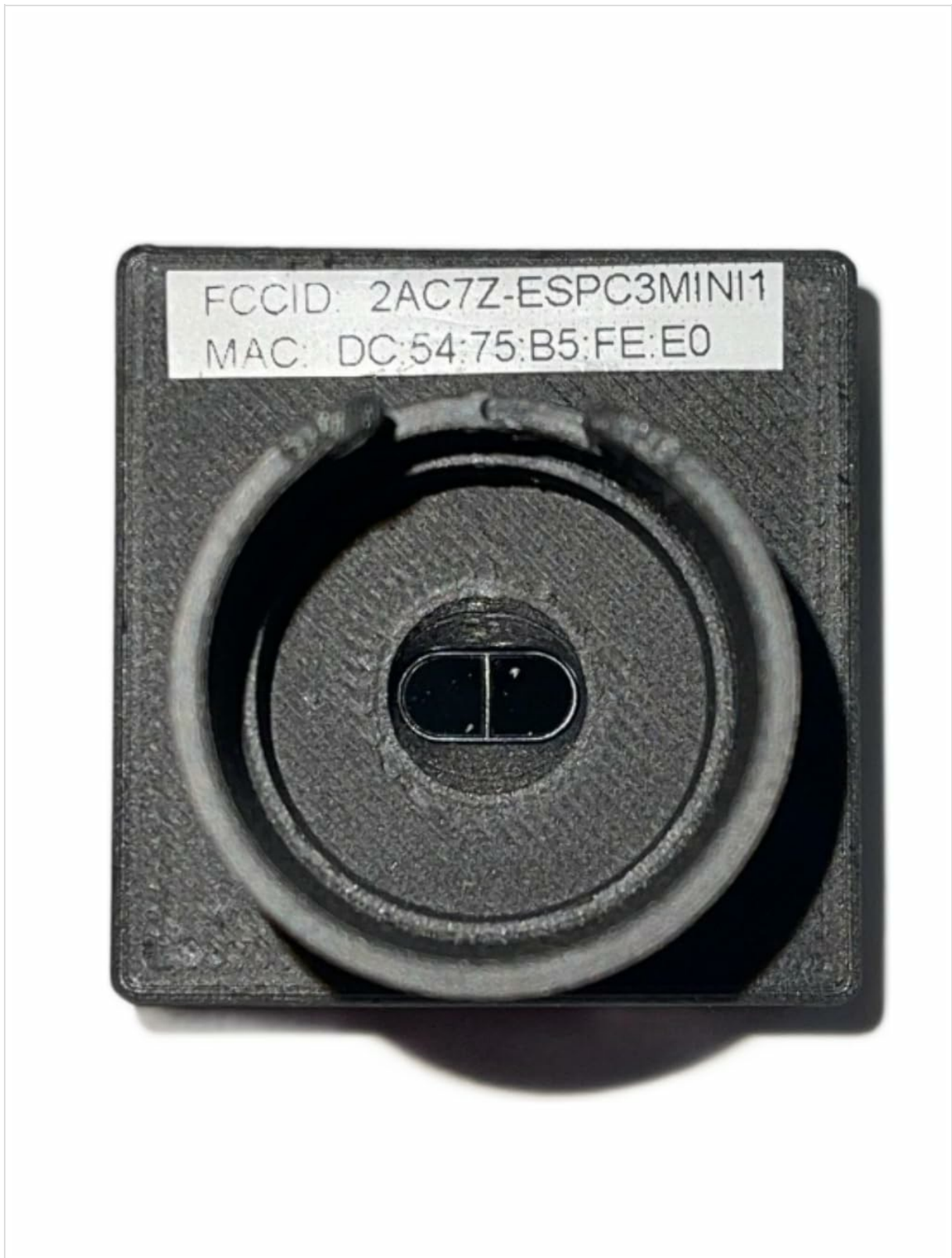
Figure 4.1: Front View of Smart Meter Unit. This image displays the front of the AVLIS-CO 2AC7Z-ESPC3MINI1 Smart Meter. Visible on the top surface is a label indicating the FCC ID: 2AC7Z-ESPC3MINI1 and MAC address: DC:54:75:B5:FE:E0. The central part features a circular opening with an internal component, likely a sensor or connection port.
