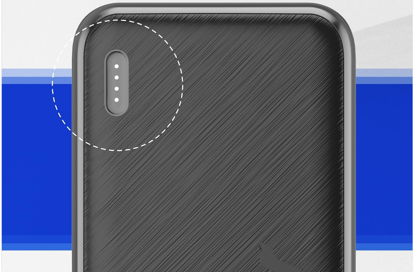
Figure 2: LED Battery Life Indicator. This image highlights the four small LED lights on the power bank, which indicate the current battery level and charging status.
