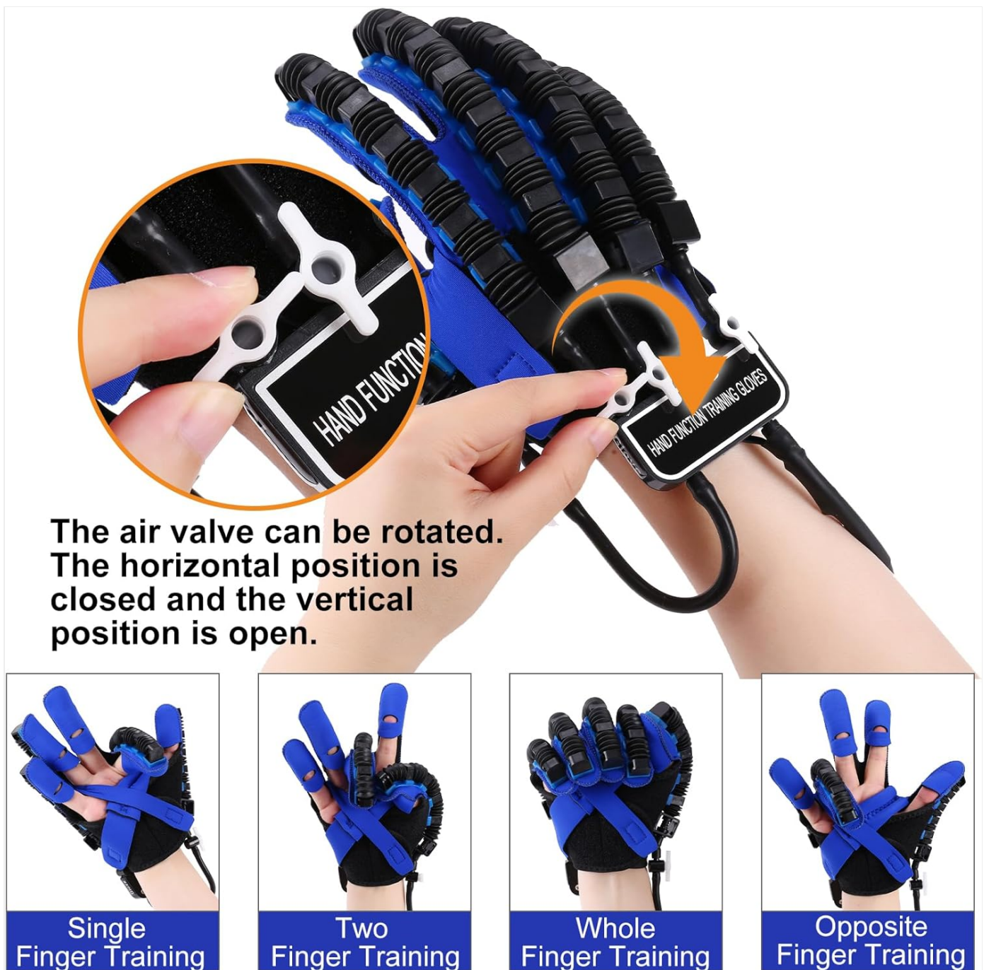
Figure 7: Adjusting air valves for specific finger training.
