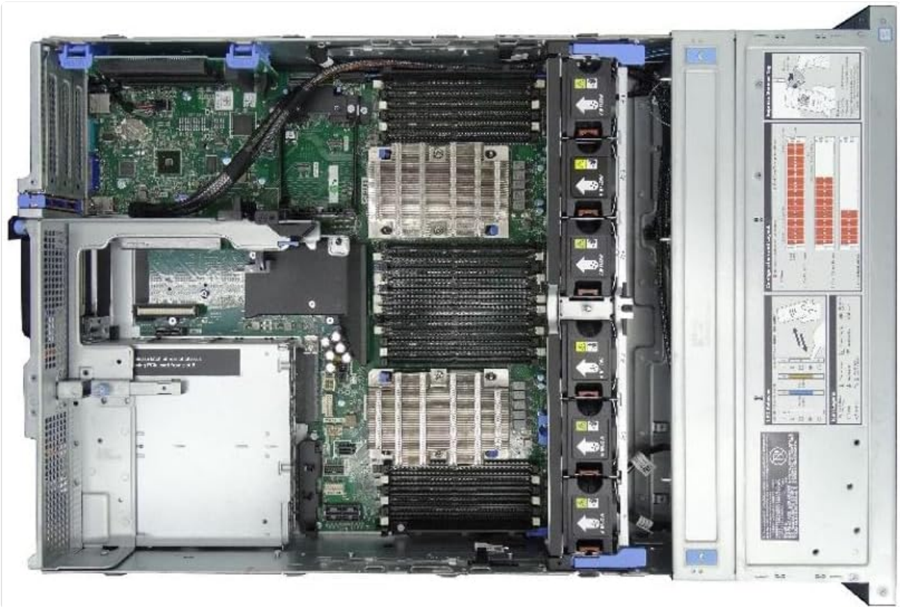
Figure 2.4: Internal view of the server, highlighting memory and storage areas.
