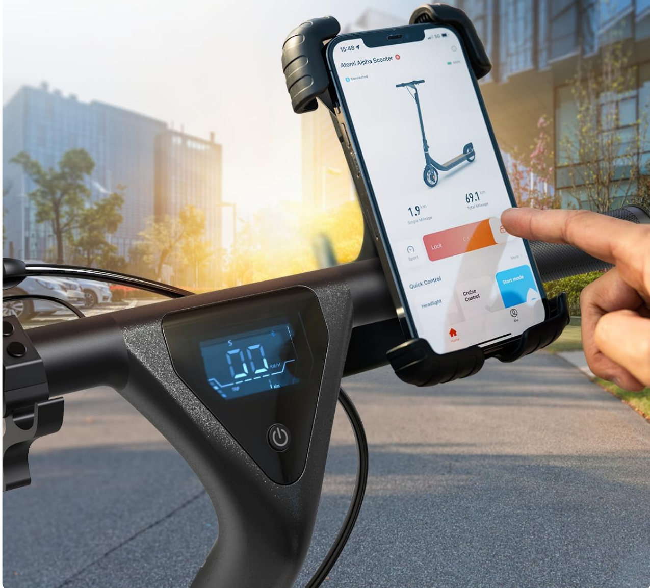
Figure 4.3: The LCD display dashboard and the smart app interface for comprehensive control.
