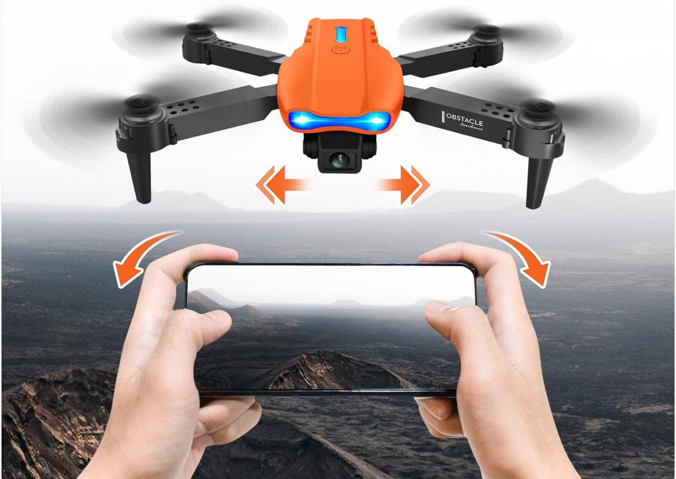
Image 6.2: The OBABO E99 Drone illustrating gravity sensing control, where the drone's movement is controlled by swinging or tilting a smartphone.
