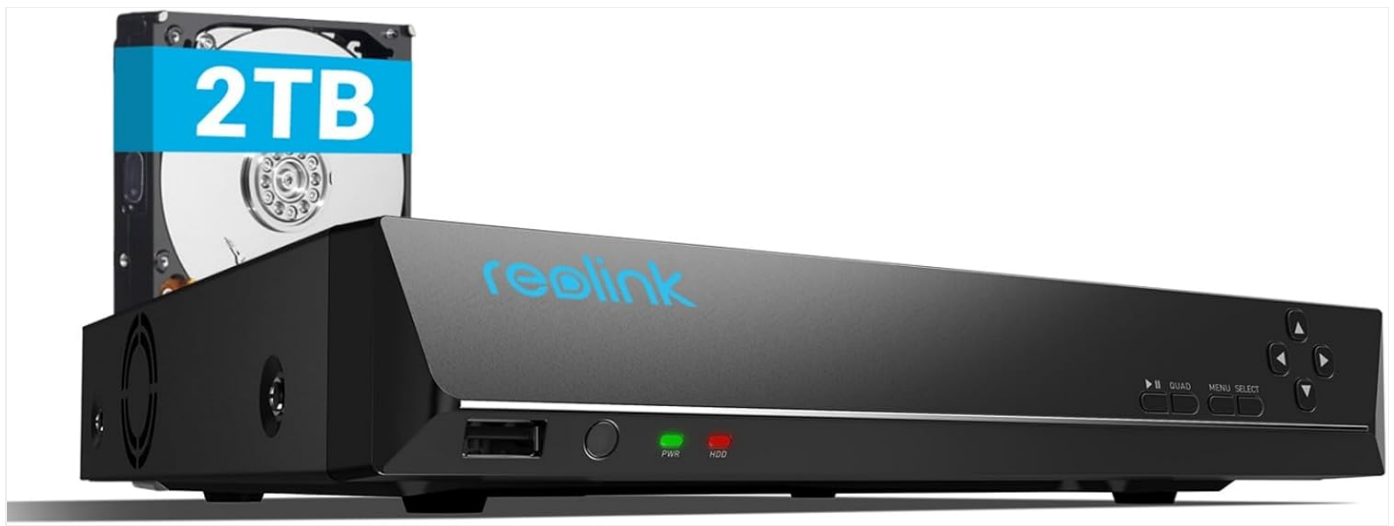
Image 3.2: The REOLINK RLN8-410 NVR unit, indicating its 2TB pre-installed hard drive.
