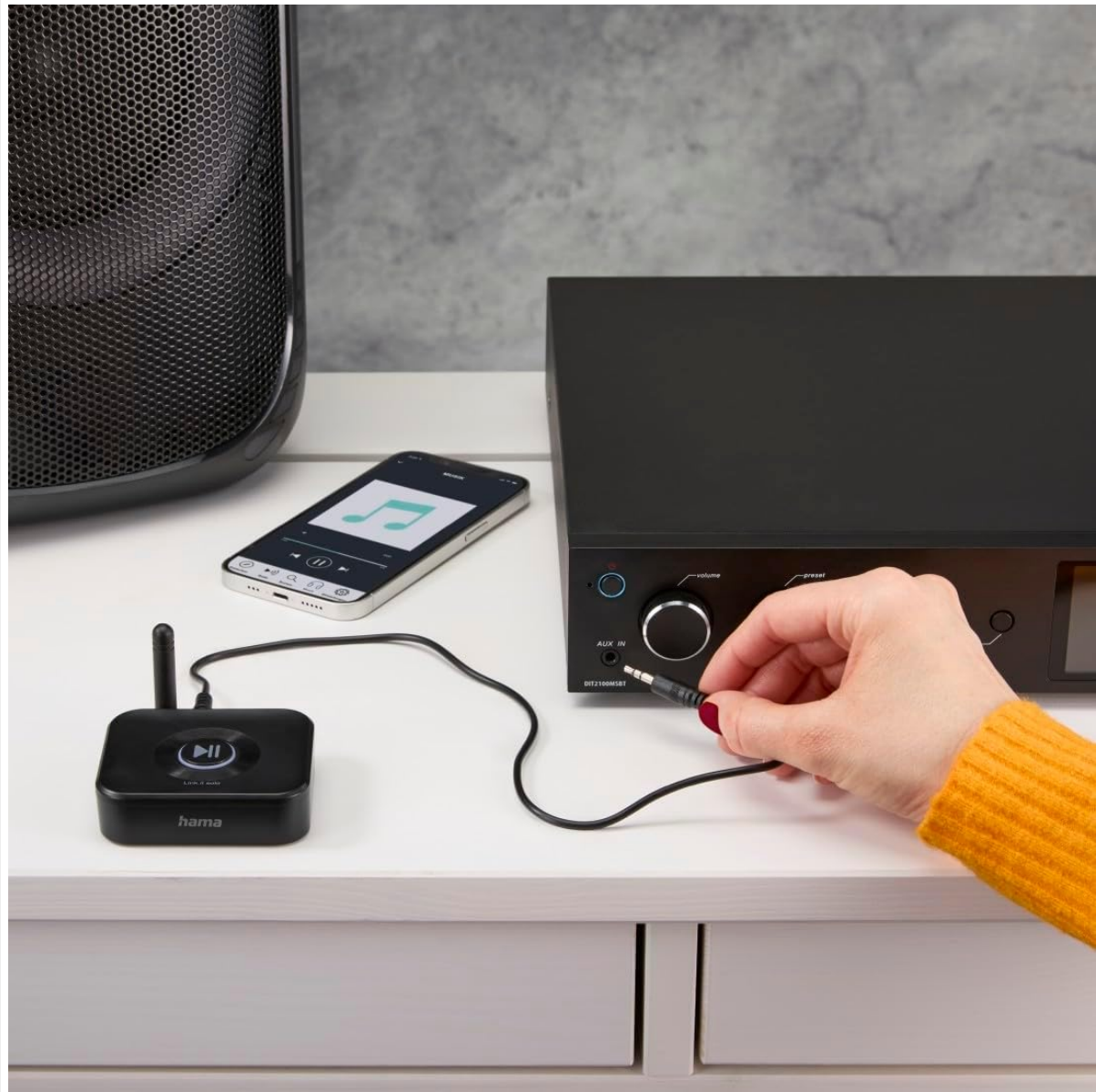
Image: A user connecting the 3.5mm audio cable from the Hama Bluetooth adapter to the AUX input of a stereo receiver, demonstrating the audio connection setup.
