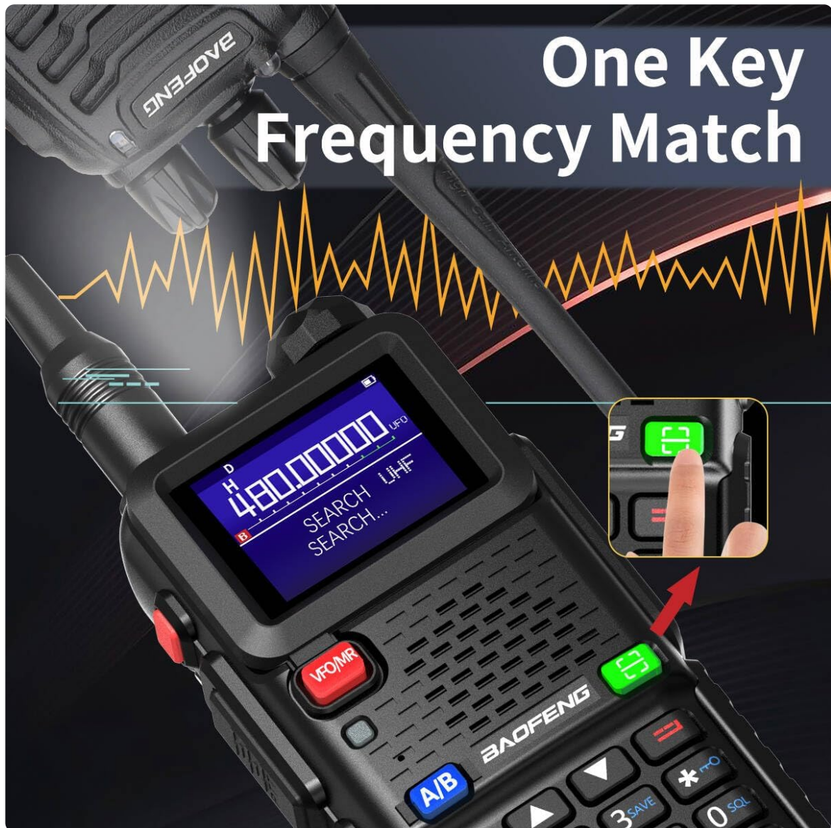
Image: A close-up of the BAOFENG AR-5RM radio showing the 'One Key Frequency Match' feature in action, indicating its ability to search and copy frequencies.
