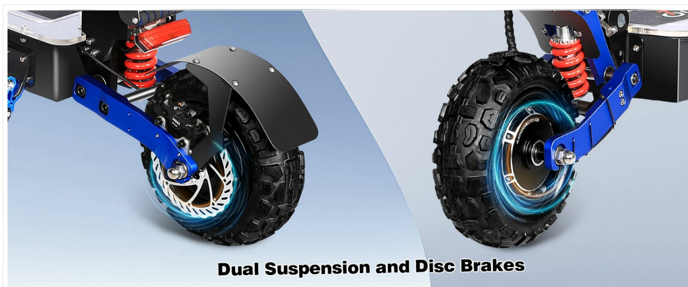
Figure 5.3: The scooter's spring damping suspension system, designed to absorb shocks and provide a smoother ride.
