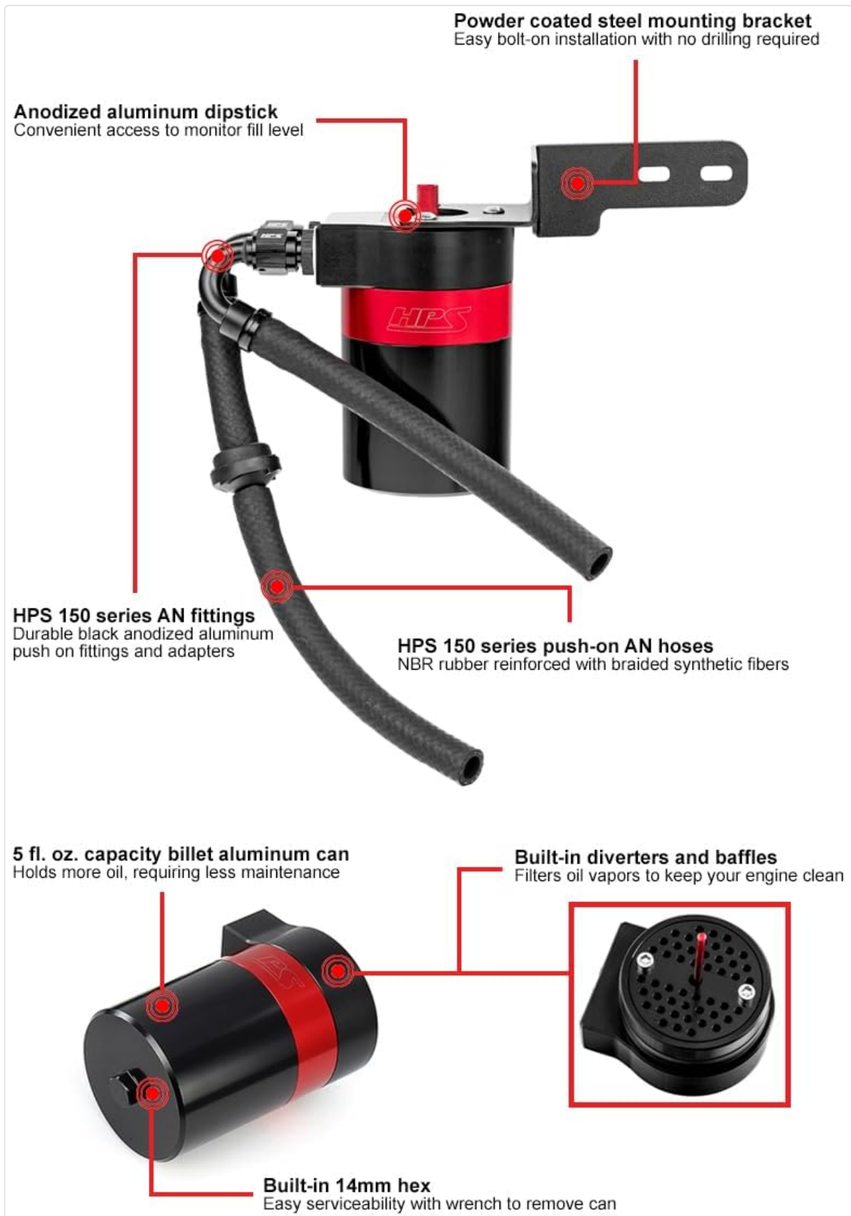
Figure 1.1: Detailed diagram illustrating the key features of the HPS Oil Catch Can Kit, including the anodized aluminum dipstick, powder-coated steel mounting bracket, AN fittings, push-on hoses, 5 fl. oz. capacity billet aluminum can, built-in diverters and baffles, and the 14mm hex for serviceability.
