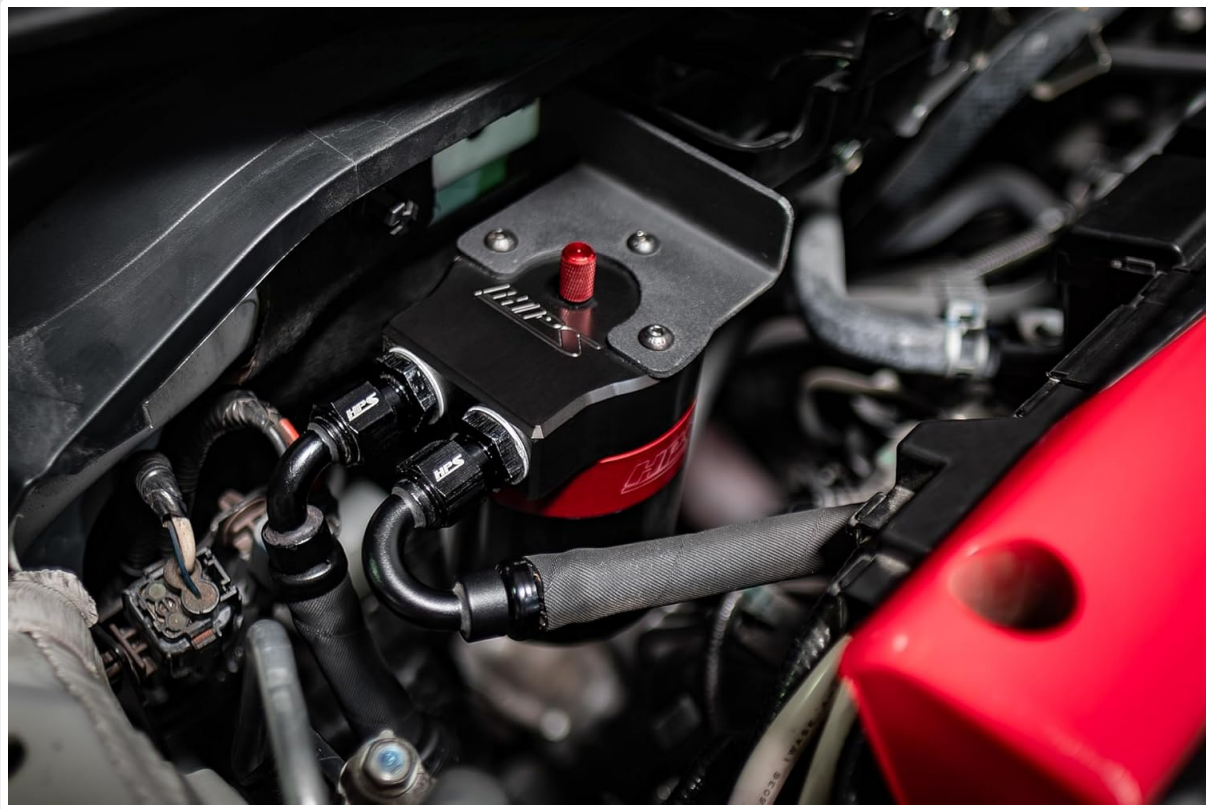
Figure 3.2: A closer view of the HPS Oil Catch Can Kit installation, highlighting the connections and mounting bracket within the engine compartment.
