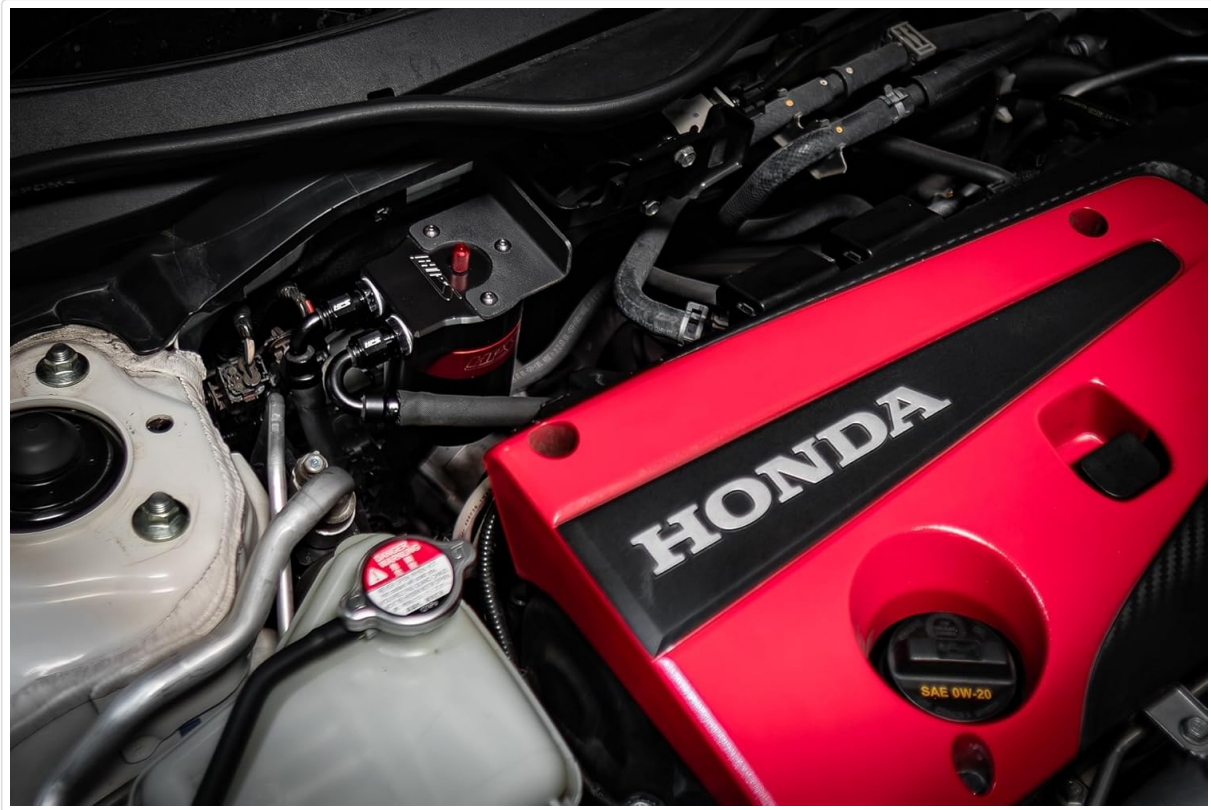
Figure 3.1: The HPS Oil Catch Can Kit installed within the engine bay of a compatible vehicle. This image shows the catch can mounted on the firewall with hoses connected to the PCV system.
