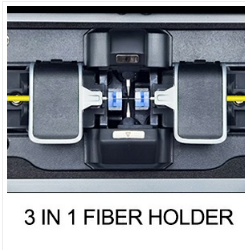
Figure 5: The 3-in-1 fiber holder for various fiber types.
