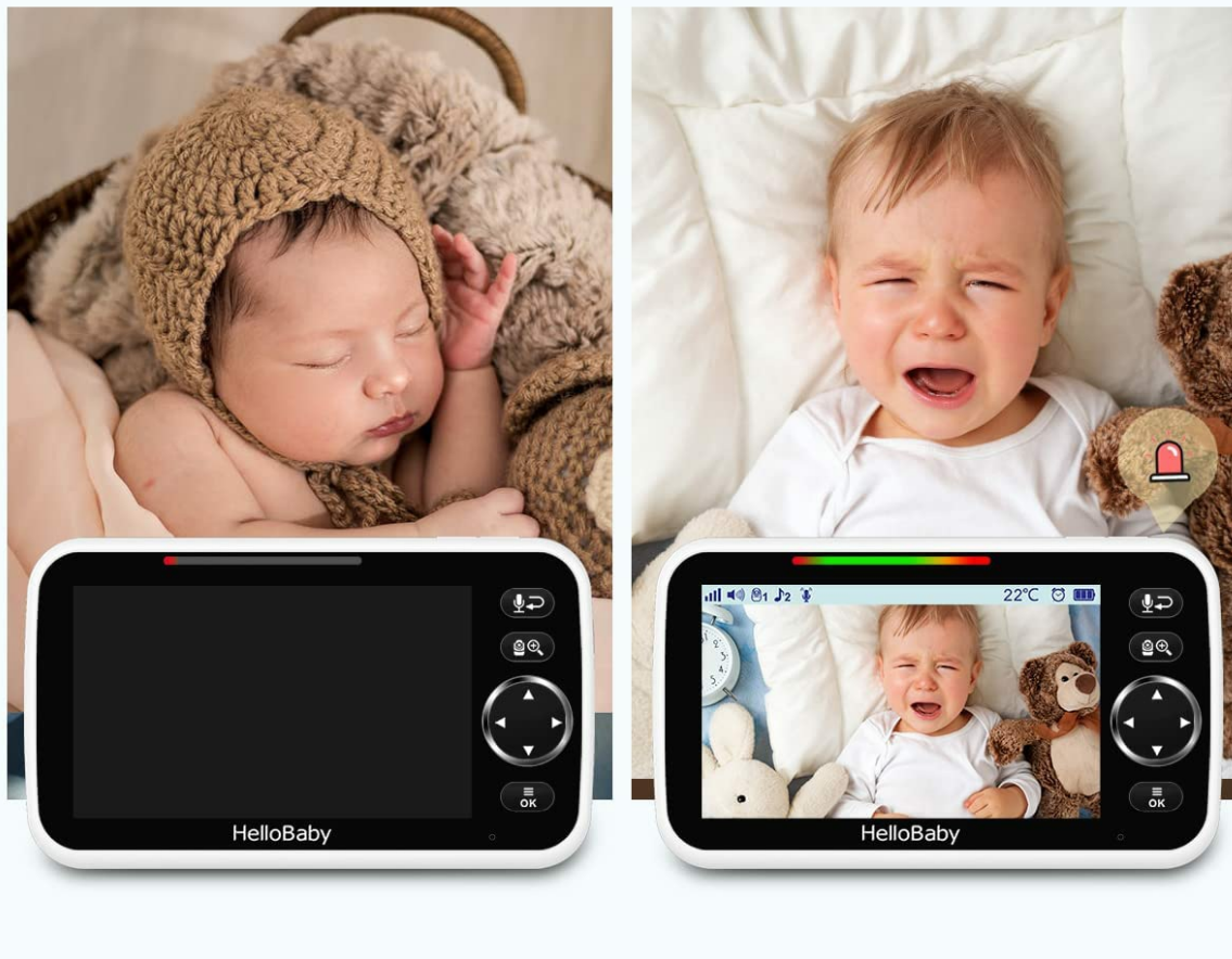
Image: Two views of the parent unit illustrating the VOX mode: one with the screen off when no sound is detected, and another with the screen on when the baby is crying.
